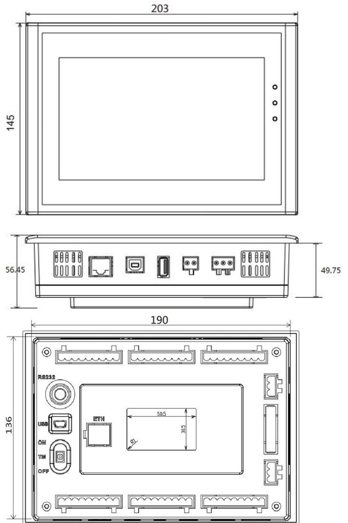
The rounded port on the left side is a port for downloading. Elliptic port is the mode selection switch, providing three options: ON, TM, and OFF. For details about ports on the right side, see port description.
