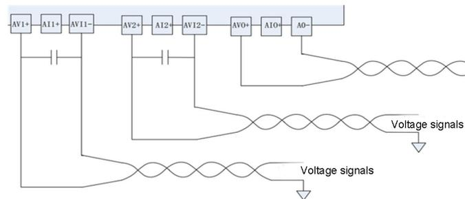
1. For analog input, it is recommended to use shielded twisted-pair cables. The cable should be kept away from the power wire or other wires that may cause electrical interference.
