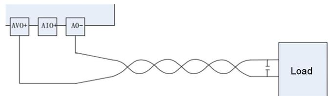
1. For analog output, it is recommended to use shielded twisted-pair cables. The cable should be kept away from the power wire or other wires that may cause electrical interference.
