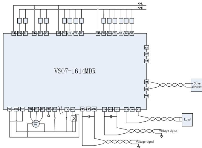
Input connection instance of analog signal
